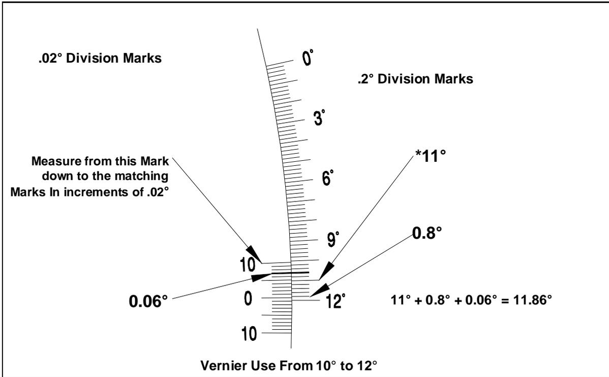
**Figure 11 Aiming, Vernier Scale**
