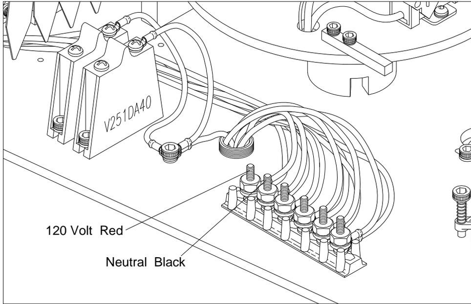
**Figure 12 Voltage Test Positions**
