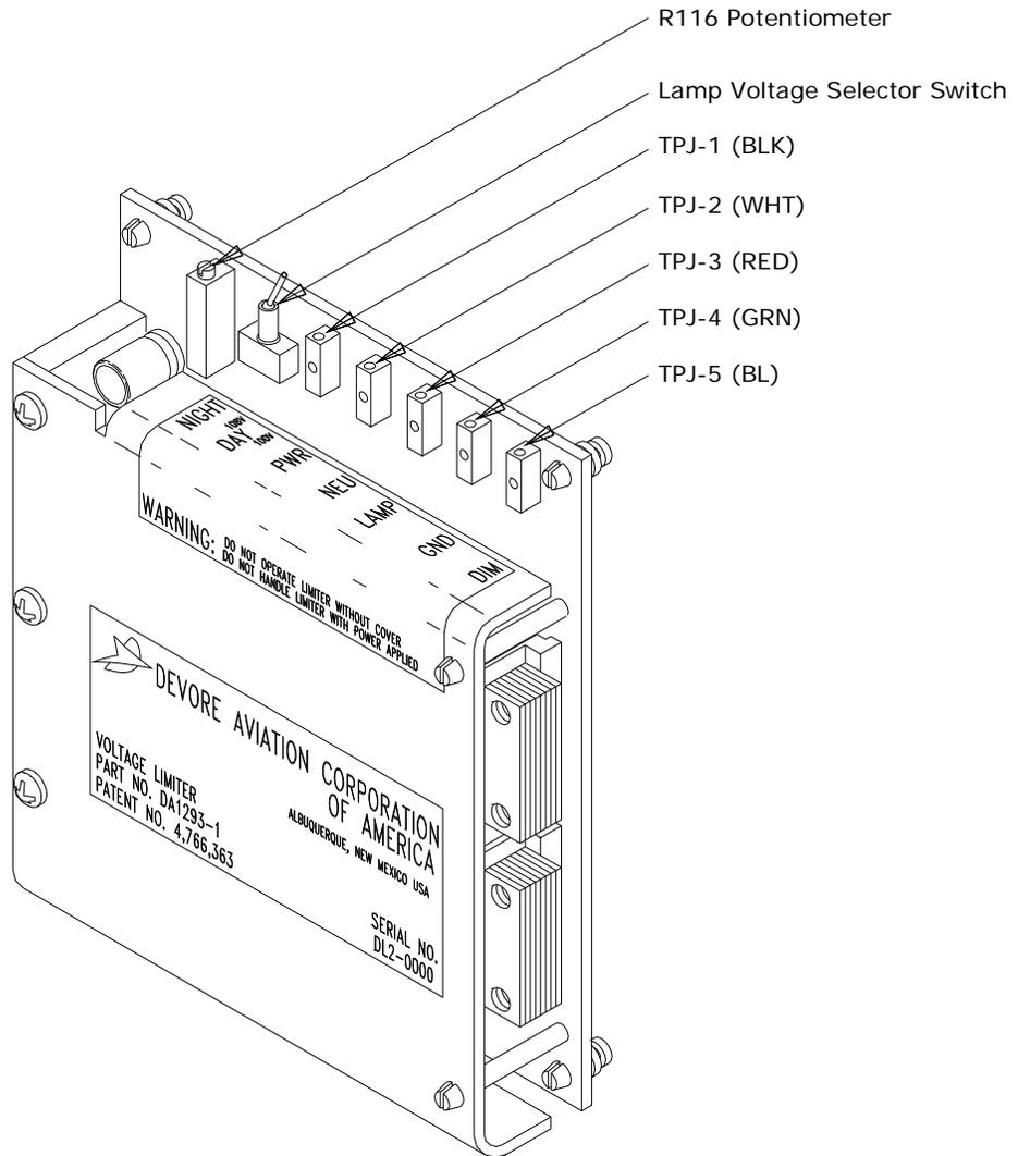
**Figure 5a Voltage Limiter**
