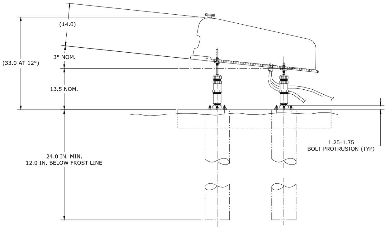
**Figure 6 PLASI 2000 System Installation (Pad Mount)**
