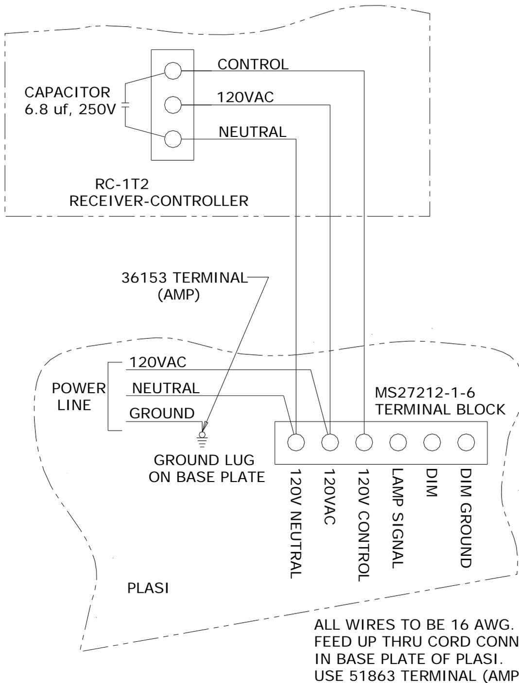
**Figure 17 Interconnect Diagram-PLASI to Radio Receiver Controller**
