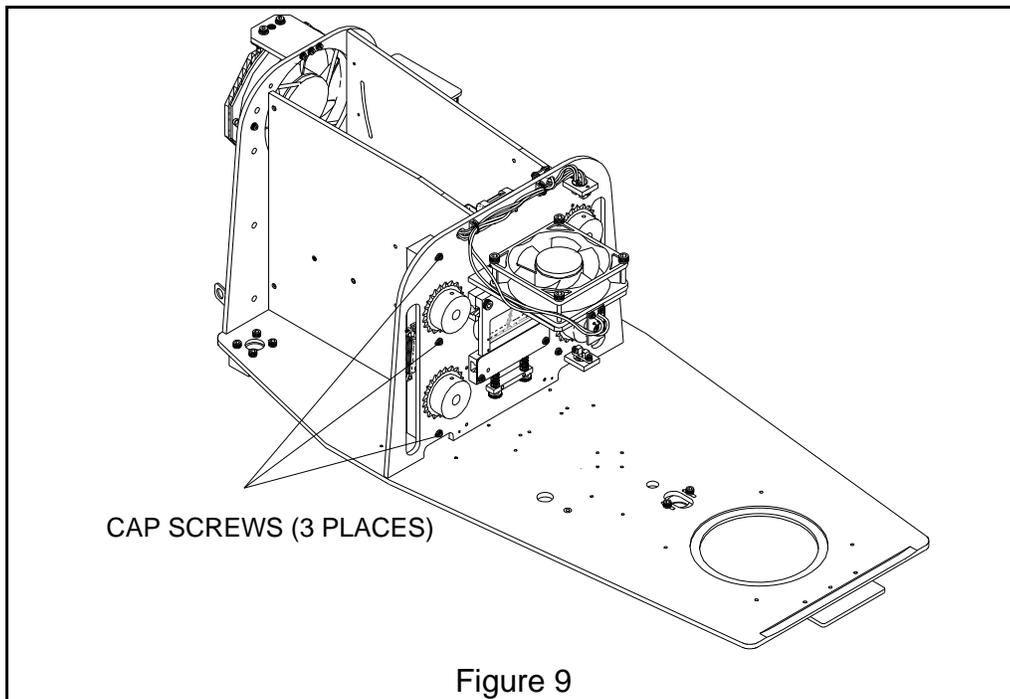
3. Move the Bearing Block Assembly to tension the chains. Both upper and lower chains must be tensioned together.
